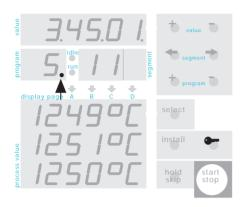
To avoid unauthorized use, you can lock the keyboard of the controller after the programme is started. Only the key (6) is still operable to call up values.
