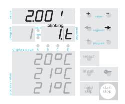
Now, enter the values for segment 1. Press the key (4) to the right hand side key once to step to the next segment (display (2) shows segment number 2).
